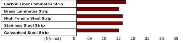
Lap Shear Strength Versus Tropical Weathering (Typical Average Values) Cure: 16 hours at 40 °C, tested at 25 °C
